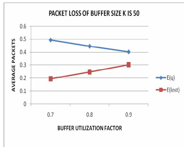
Fig. 4: Packet Loss as a function of Buffer size is 50
