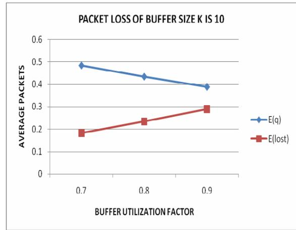
Fig. 3: Packet Loss as a function of Buffer size is 10
