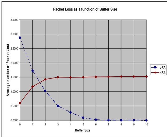
Fig. 2: Average Packet Loss as a function of Buffer Size
